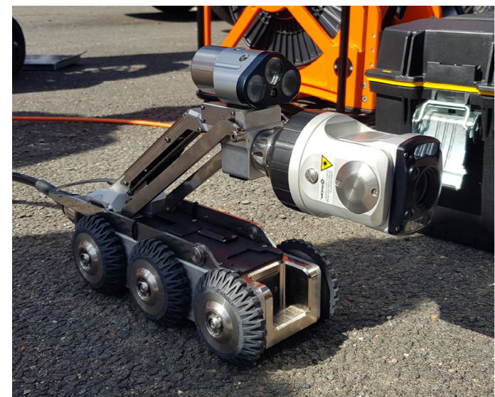
Above: one of our state-of-the-art CCTV drain survey cameras with front mounted pan & rotate zoom and high powered ultra-bright LED lighting, allows us to map drains and inspect faults in incredible detail, even when obstructions block the way.
